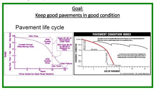
The goal is to extend the life of the pavement. Doing these repairs on the pavement can save money in the long term. A dollar spent today and save four to five dollars in maintenance. Chuck explained that PCI is only one factor used when determining street maintenance needs. They look at traffic volume, speed, safety, road classification, affordability and location.
