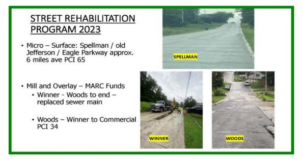
Chuck explained that the 2023 proposed budget includes \$300,000 for the mill and overlay program. In it staff is recommending that Spellman Drive, Old Jefferson Highway and Eagle Parkway, approximately six miles long and the PCI average is 65 receive a micro-surfacing treatment. He noted that if we repair the road now it would be more cost effective and extend the life of that road.
